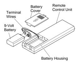
Figure 48 - Installing Battery in Hand-Held Remote Control Unit
